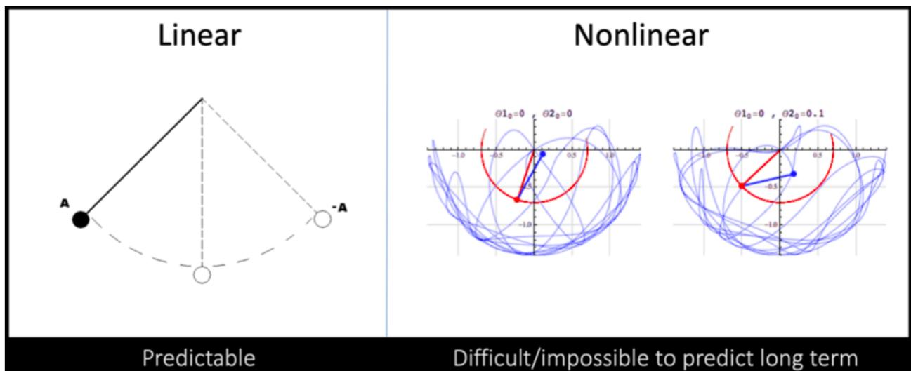
A simple pendulum (linear system) on the left swinging back and forth; and two double pendulums (nonlinear systems) to the right, one with a slightly different starting position to the other.
